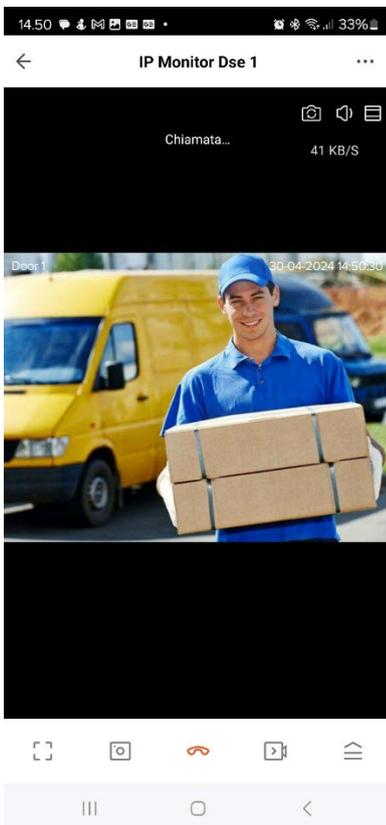
To open the door, open the full toolbar and choose LOCK. You can act on 2 buttons which they control the 2 locks connected to the pushbutton panel.
